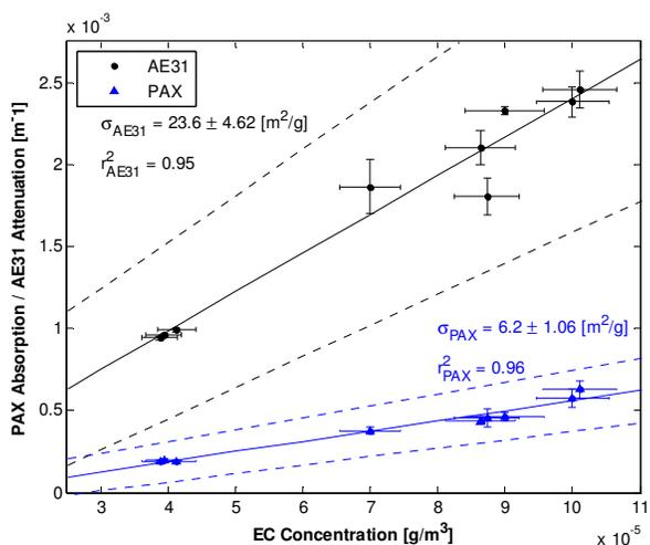
Figure 6: Aerosol Absorption and Attenuation vs NIOSH 5040 EC Concentration. Dashed lines represent the 95% confidence interval on the linear fit.
