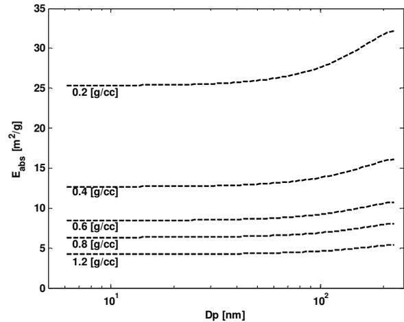
Figure 1: Mass specific particle absorption efficiency for diesel soot
