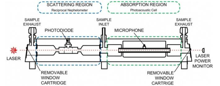
Figure 3: Schematic of DMT PAX Acoustic chamber [23]
