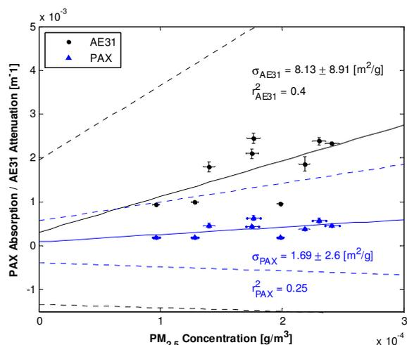
Figure 7: Aerosol Absorption and Attenuation vs.  $PM_{2.5}$  Mass Concentration. Dashed lines represent the 95% confidence interval on the linear fit.
