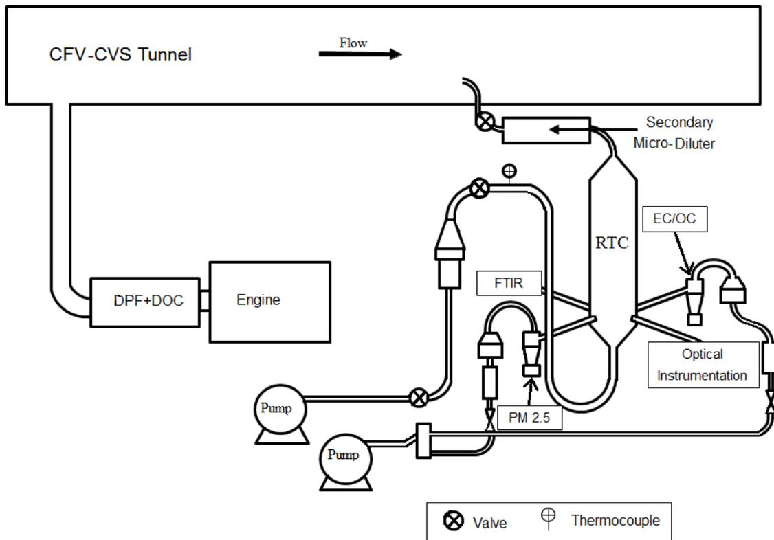
Figure 2: Test Cell and Dilution System Schematic
