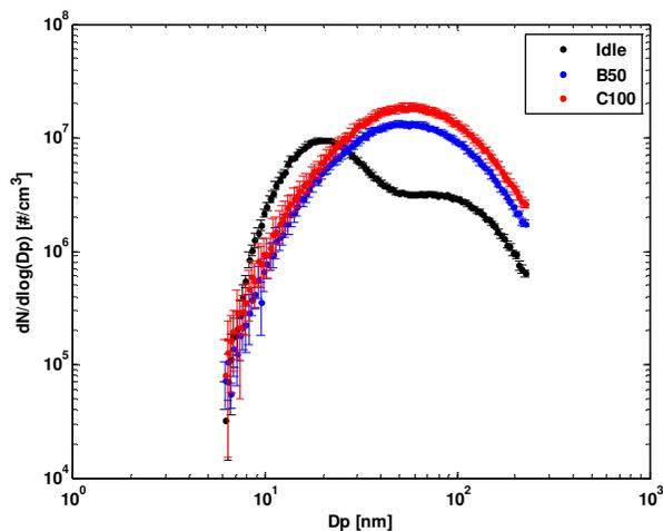
Figure 5: Particle Size Distributions for each engine mode
