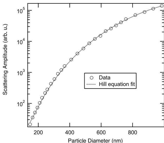
**Figure 4.** Scattering amplitude of dioctyl sebacate aerosol versus size as measured with the SP2. The aerosol was size selected with an electrostatic sorter. The fitting function was a Hill equation.
