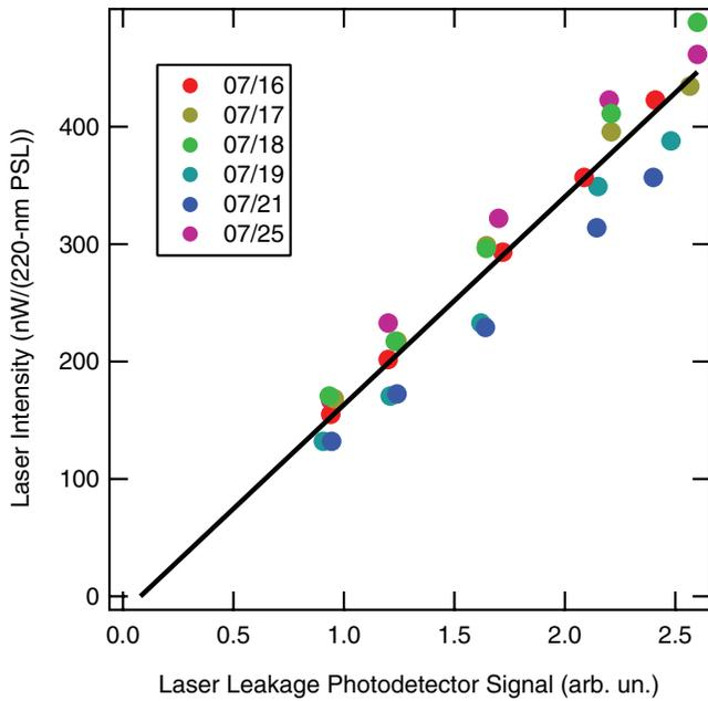
FIG. 3. Comparison of the measurement of laser intensity based on measurements inside and outside the cavity. The latter is measured with the laser leakage photodetector. The former is measured as the most probable peak power incident on the SP2 scatter detector when a polystyrene latex sphere (PSL) of known diameter and index of refraction is sampled (see text). The power in the laser cavity was varied by changing the amount of pump laser light incident on the Nd:YAG crystal.
