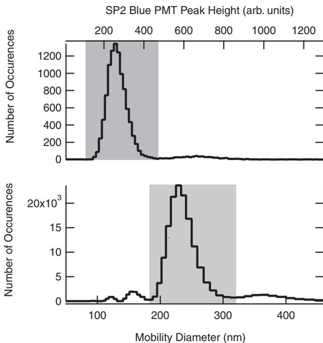
FIG. 4. Top: SP2 peak height distribution for typical sample of FGS aerosol used to in the analysis here. Bottom: the SMPS distribution for the same FGS sample. The shaded sections represent the selected peak height and diameter ranges, respectively, for the primary aerosol mode for which SP2 detection efficiency was calculated.
