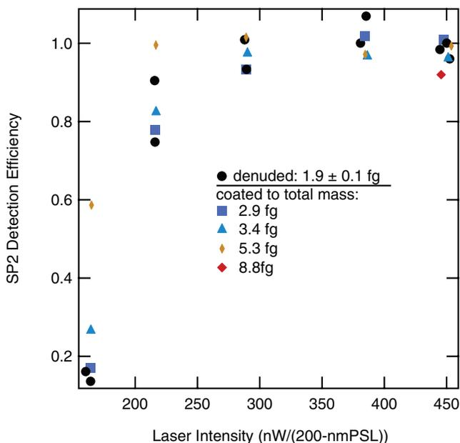
FIG. 10. Average SP2 detection efficiency for FSG generated with an equivalence ratio ( $\phi$ ) of 1.9, size selected with a DMA, and then coated with increasing thicknesses of sulfuric acid. The total-particle masses of the denuded rBC-core particles and coated particles as noted in the legend were determined with the CPMA. The denuded core mass was  $1.9 \pm 0.1$  fg. Particles were sampled at 1000 hPa.
