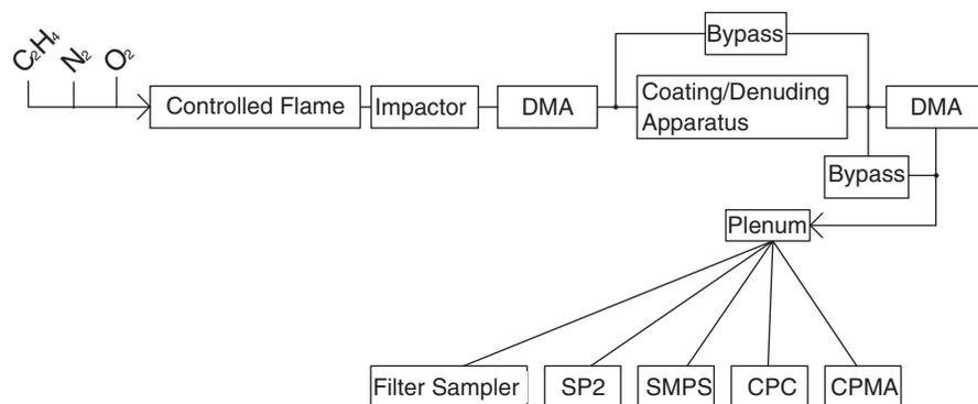
FIG. 1. Schematic of the flame-generated soot generation and detection scheme with the filter sampler, single particle soot photometer (SP2), scanning mobility particle sizer (SMPS), condensation particle counter (CPC), Couette centrifugal particle mass analyzer (CPMA), and differential mobility analyzer (DMA).
