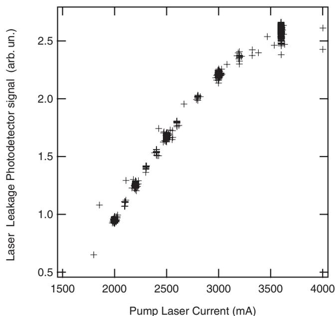
FIG. 6. Laser-cavity leakage as measured with a photodetector as a function of the current driven through the solid-state pump laser. Each data point is the value averaged over a single experimental setup and laser intensity tested ( $\sim 850$  points).
