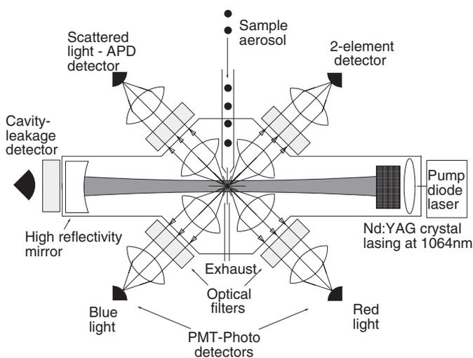
FIG. 2. Schematic of the Single Particle Soot Photometer (SP2) following Schwarz et al. (2006). The sample aerosol is confined with filtered sheath flow to the center  $1/4$  of the laser beam, and then drawn out of the laser cavity through the exhaust line. Although drawn in the page for simplicity, the sample line and exhaust lines extend perpendicular to the detection axes (i.e., vertically into and out of the page).
