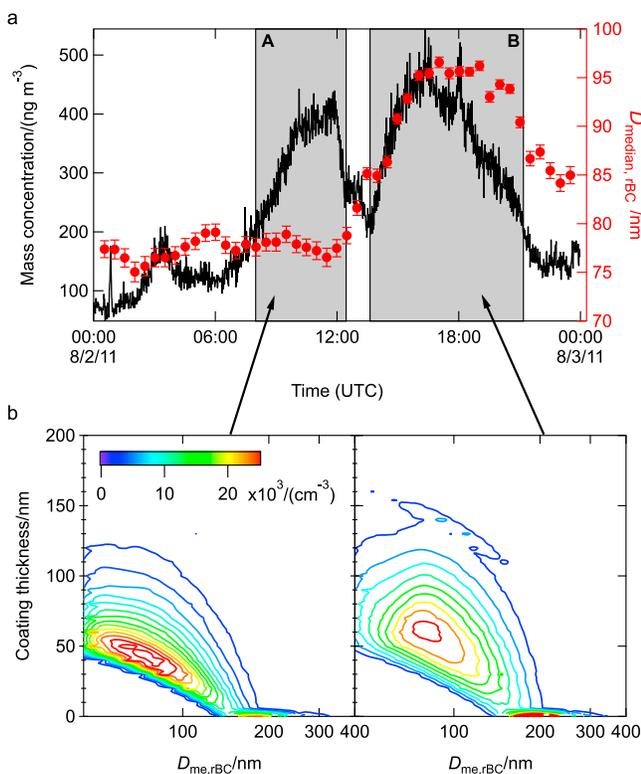
**Figure 1.** (a) Mass concentration of rBC (black line) determined by incandescence and median diameter of rBC,  $D_{\text{median,rBC}}$ , integrated over 30-min intervals (red dots) with error bars denoting one standard deviation. Shaded regions delineate episodes A and B. (b) Coating thickness of rBC-containing particles determined by optical diameter method integrated over episode A and B as a function of rBC mass-equivalent diameter,  $D_{\text{me,rBC}}$ .
