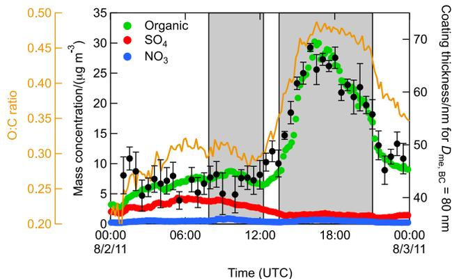
**Figure 2.** Aerosol mass concentration of organics (green),  $\text{SO}_4$  (red), and  $\text{NO}_3$  (blue), with O:C ratio (gold), all determined by the High Resolution Time-of-Flight Aerosol Mass Spectrometer (HR-ToF-AMS), and coating thickness determined by the optical diameter method of rBC-containing particles with  $D_{\text{me,rBC}} = 80$  nm (black), with error bars denoting one standard deviation. Shaded regions delineate episodes A and B as in Figure 1.
