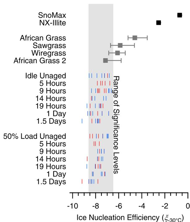
**Figure 2.** Ice nucleation efficiency of diesel (red sticks) and biodiesel (blue sticks) exhaust under idle and 50% load conditions. Also shown are time-averaged data for laboratory burns of biomass fuels from FLAME4 [Levin *et al.*, 2016] (dark grey markers) and from 500 nm size-selected SnoMax and NX-illite particles (this study; black markers). The range of significance for all diesel-exhaust sampling periods is highlighted in grey.
