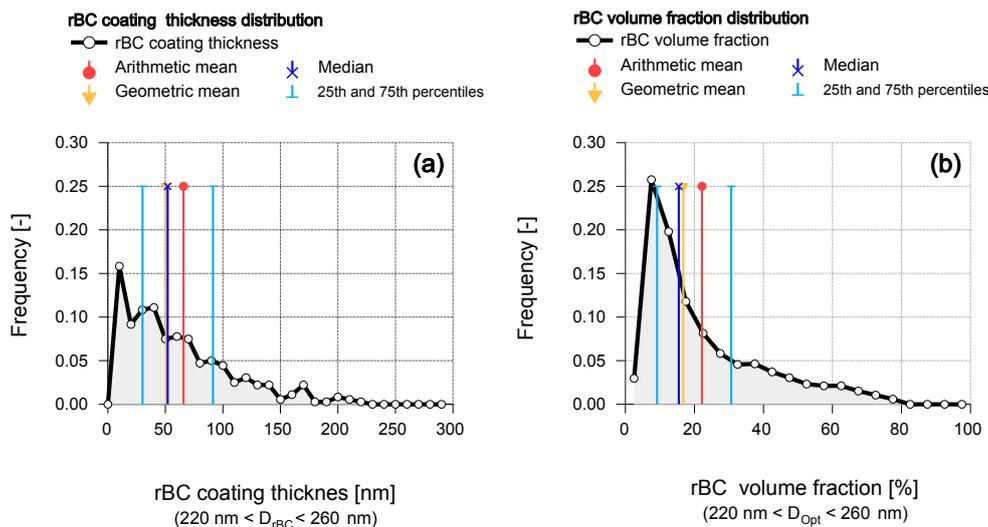
**Figure 4.** Frequency distributions of single-particle properties inferred from the SP2 measurement during the whole campaign: **(a)** BC coating thickness of BC cores with  $220 \text{ nm} < D_{\text{rBC}} < 260 \text{ nm}$ ; **(b)** rBC volume fraction distribution of BC-containing particles having an optical diameter between 220 and 260 nm.
