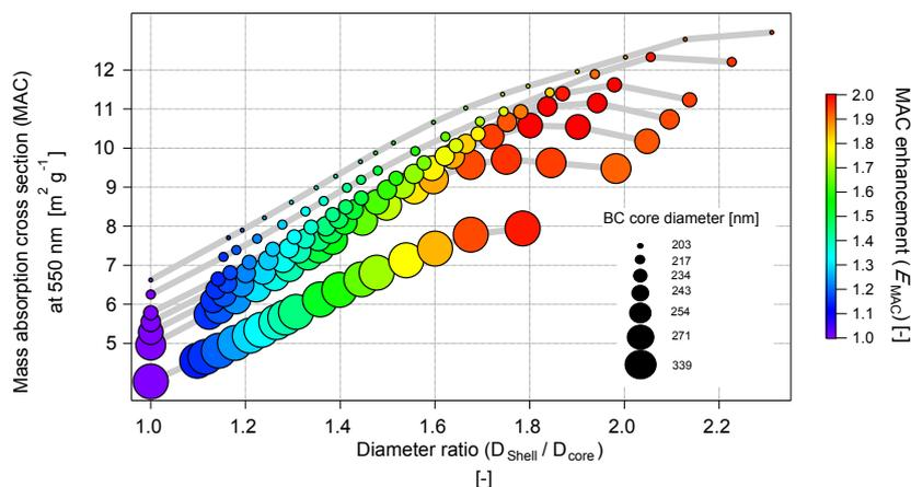
**Figure 6.** Mass absorption cross section ( $\text{MAC}_{\text{Mod}}$ ) of BC-containing particles calculated according to Mie theory as a function of its mixing degree and BC core diameter assuming a core–shell mixing geometry. MAC enhancement ( $E_{\text{MAC}}$ ) is defined as the ratio of the MAC of a coated BC core divided by the MAC of the same BC core without coating.
