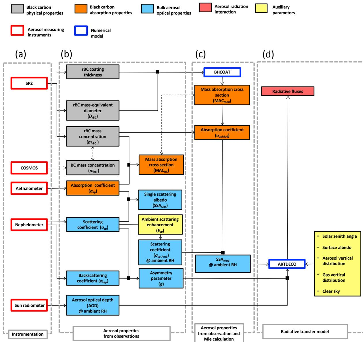
**Figure 1.** Flow chart from observations to radiative forcing: (a) deployed instruments; (b) observed properties; (c) properties obtained from optical model constrained by observations; (d) radiative transfer model simulations. Measurements and quantities are generally for low RH (“dry”), unless “@ ambient RH” is explicitly stated.
