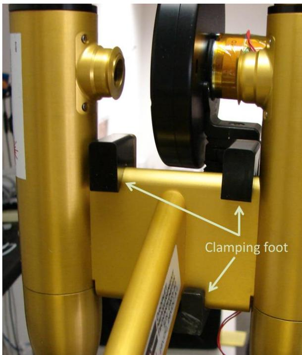
*Figure 1: Spinning Pinhole Mounting Clamp*
