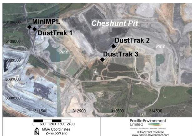
Figure 3. Lidar and PM monitor locations at Cheshunt Pit, HVO
