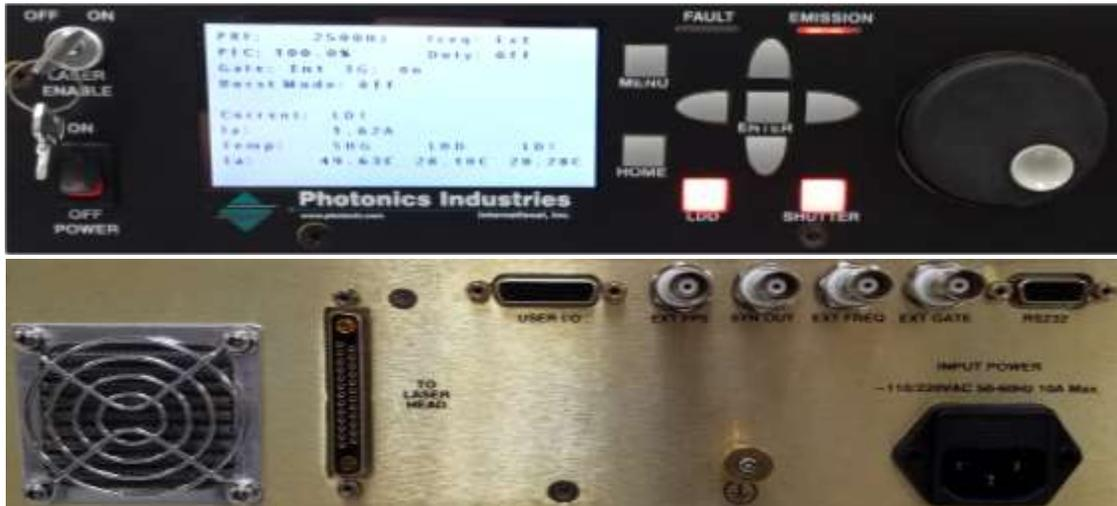
Figure 2: Laser Power Supply Front and Rear Panels
